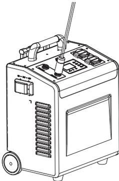
**Figure 11** UBird-XN AC Input Wiring
