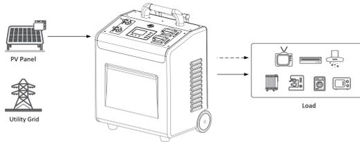
When PV power is less than the consumption, and the battery capacity is low, grid supplies the load, PV charges the battery, if there is rest PV power, supply the load.
