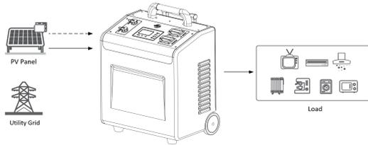
When PV power is less than the consumption, and the battery capacity is high, PV and battery supply power to the load at the same time.
